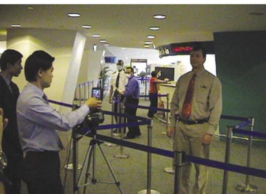
Setting up a ThermaCAM with Automatic Temperature Compensator (ATC) for viral disease detection.
