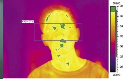
The ThermaCAM automatically detects the hottest temperature within an area, set by the operator. A color alarm makes it easy to decide whether a person needs further examination or not.
