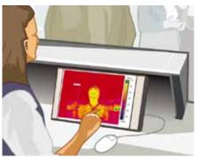
**Step 2:** IR camera operator looks at a color monitor that shows audible and/or visible color alarms when an individual shows an "out of norm" body temperature.
