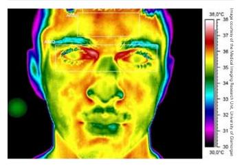
FLIR IR cameras automatically detect elevated skin temperatures that may indicate a fever and underlying infection. Each camera's unique Automatic Temperature Compensator (ATC) adjusts for ambient conditions to minimize false readings. The color image, temperature scale, and alarm mechanism make it easy to decide when a person needs further examination.
