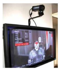
Fixed-mount FLIR A320 with the color alarming in progress
